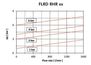
N.B. All the reported data have been obtained at our laboratory, according to specification ISO3968 with mineral oil having 32 cSt viscosity and density  $0.875 \text{ Kg/dm}^3$ .
