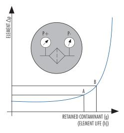
The **Pressure Drop** ( $\Delta p$  = differential pressure) through the filter increases during the system operation due to the contaminant retained by the filter element.
