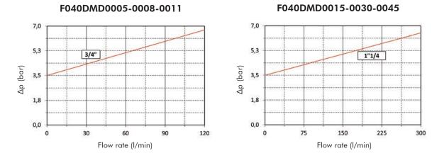
N.B. All the reported data have been obtained at our laboratory, according to specification ISO3968 with mineral oil having 32 cSt viscosity and density 0,875 Kg/dm<sup>3</sup>.
