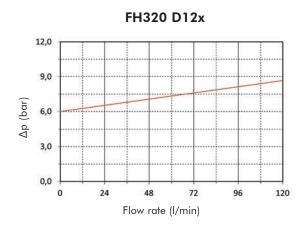
N.B. All the reported data have been obtained at our laboratory, according to specification ISO3968 with mineral oil having 32 cSt viscosity and density  $0.875 \text{ Kg/dm}^3$ .
