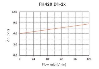
N.B. All the reported data have been obtained at our laboratory, according to specification ISO3968 with mineral oil having 32 cSt viscosity and density 0,875 Kg/dm<sup>3</sup>.
