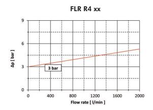
N.B. All the reported data have been obtained at our laboratory, according to specification ISO3968 with mineral oil having 32 cSt viscosity and density 0,875 Kg/dm³.
