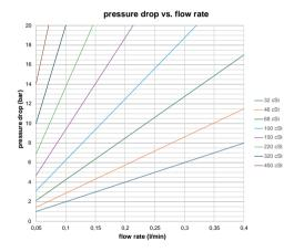
Considering the above values, Filtrec suggests using this kind of connection only for viscosity of 150 cSt or less.
