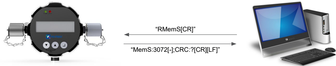
Fig. 24: Example data transmission RS232 with checksum
