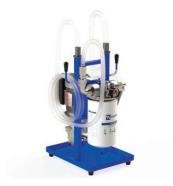
When the operation is completed, rewind the power cable, inlet and outlet hoses. Be careful when draining the oil contained in them and insert the ends of the hoses into the cases.
