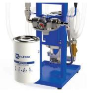
Verify the correct part number of the FILTREC replacement cartridge, particularly concerning the micron rating. Ensure that the mounting face is clean, lubricate the gasket of the replacement cartridge prior to assembly. Spin on new cartridge until it reaches the mounting face and tighten for 3/4 turn.
