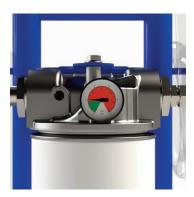
The inline filter has a clogging indicator (pressure gauge), the cartridge must be replaced when the pointer reaches the red sector.
