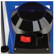
Push the button on "0" when the operation is finished.
